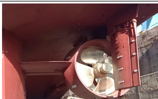
Foto 13 – Propulsor principal (boreste)
